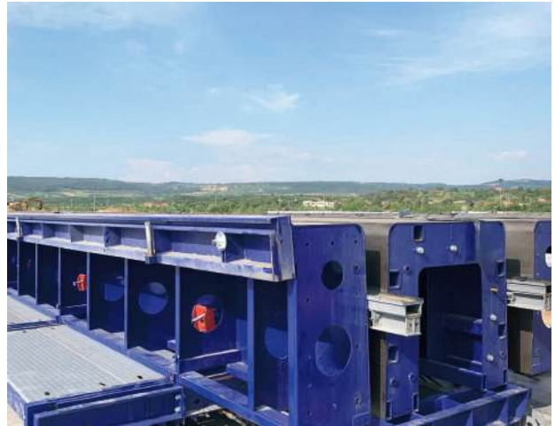
Mould with hydraulic opening and hydraulic rib height adjustment.
