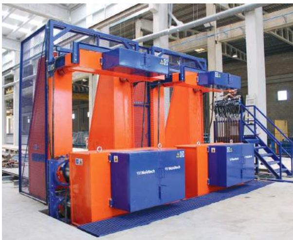
Lower and upper drill matrix with safety system.
