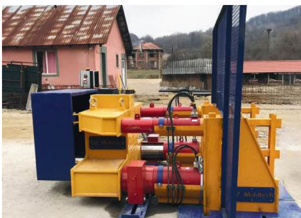
Lower and upper drill matrix with safety system.
