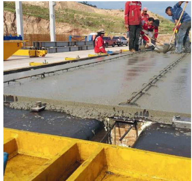
Mould with hydraulic opening and hydraulic rib height adjustment.
