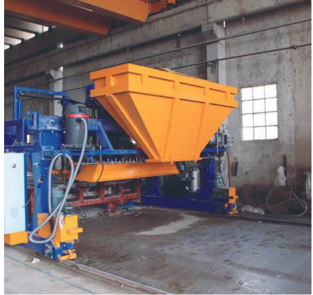
Casting bed cleaning machine.
